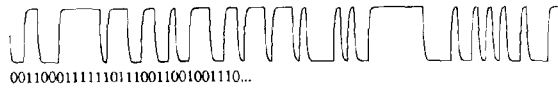
Fig. 2. Illustration of a digital signal with a finite rise-time as generated by an RC time-constant, where the Boolean signal abstraction is shown below.
