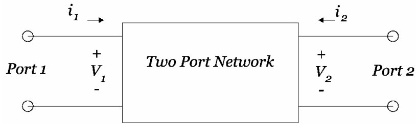
Figure 2.1. Two-port network diagram
