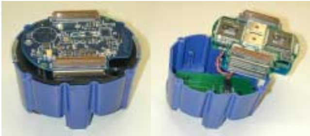
Figure 1: A fully assembled Test Bed node with sensor board, and a case with the core boards and radio board removed
