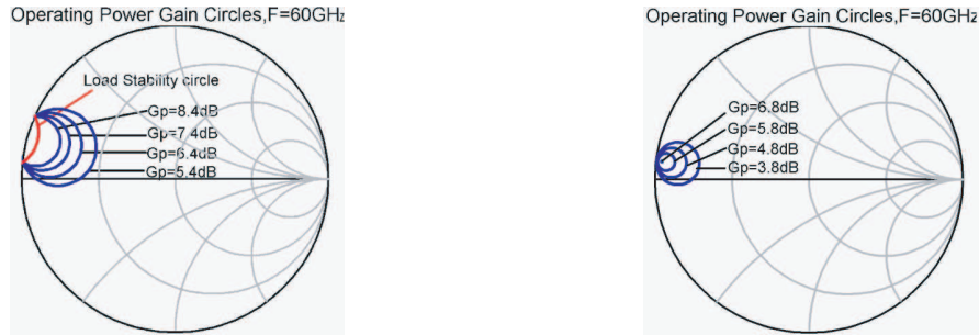
Fig. 3. Load impedance contours of power gain for the 2\ \mu (left) and 4\ \mu (right) device.
